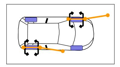
o If, due to motor vehicle safety reasons, anchoring is impossible by using two chocks per wheel, it is necessary to use 4 chocks to fasten 4 wheels of motor vehicle.
