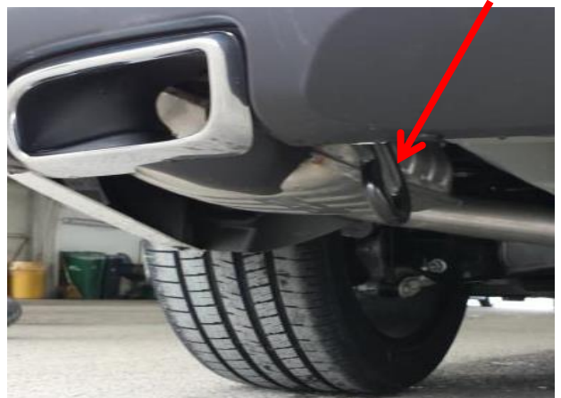
Wheel lash in rear, except on the Chrysler 300 which has a fixed loop
