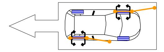
If, due to motor vehicle safety or technical reasons, anchoring is impossible by using two chocks per wheel, it is necessary to use 4 chocks to fasten 4 wheels of motor vehicle.
