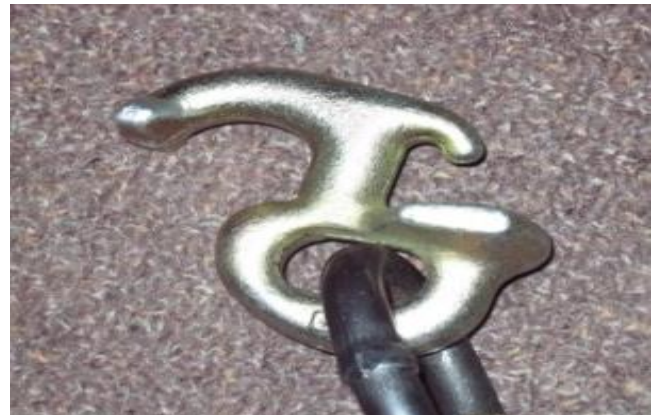
Hard Tie – Chains – R Hook Only
